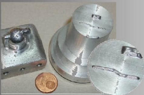
High alloy aluminium applied using laser welding
