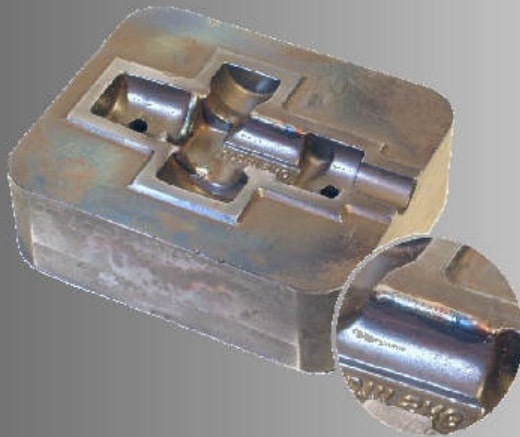
Hot work tool repaired with CRONITEX - SUPERPLUS - for a longer structure lifetime. Filler metal Rc 60
