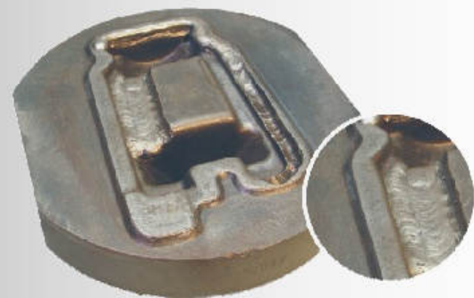
Worn areas of the forging die are gouged, cracks are joined with CRONITEX electrode 252-C and then build-up welded with CRONITEX electrode Multiloy.
