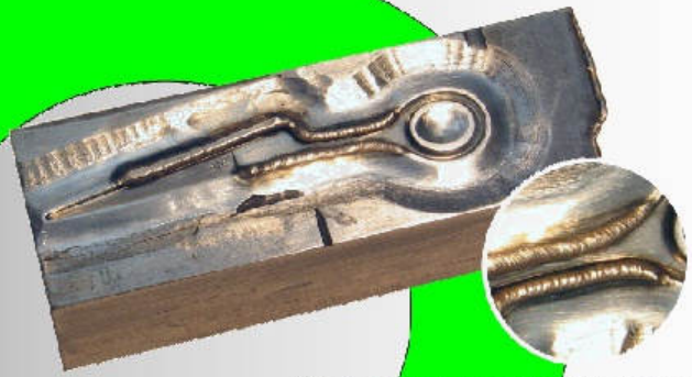
Worn out shear die saved through repair welding
